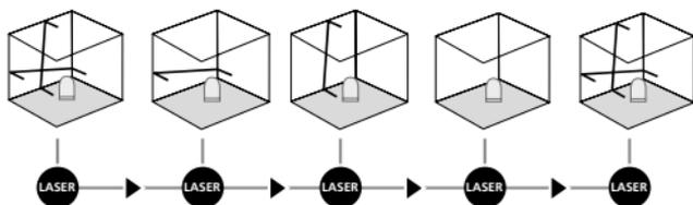
Do not release the transport restraint, set the ON/OFF switch to „OFF“. Select and switch on the laser with the selection button. Sloping planes can now be measured. This mode cannot be used to perform horizontal or vertical levelling as the laser lines are no longer aligned automatically. The LED (2) lights constantly red.
