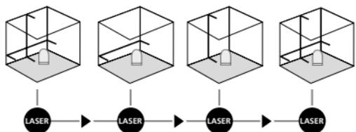
**!** The transport restraint must be released for horizontal and vertical levelling. The LED (2) shows a permanent green light. The laser lines flash and the LED (2) lights red as soon as the device is outside the automatic levelling range of 5°. Position the device such that it is within the levelling range. The LED (2) switches back to green and the laser lines stop flashing (steady light).
