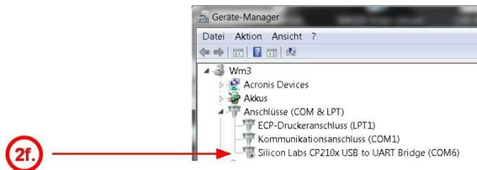
2f.) After install the new COM port must be available in the System\Hardware dialog.
